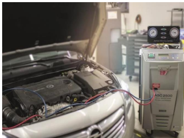
Refrigerant refill. Source: ADAC Air Conditioning Service
